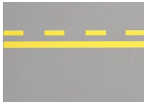
Non-Movement Area Solid side indicates area NOT under ATC control
